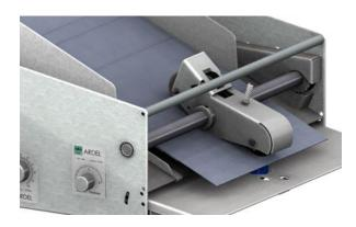
Place the load so that the drive wheel is in contact with the first product to feed.
