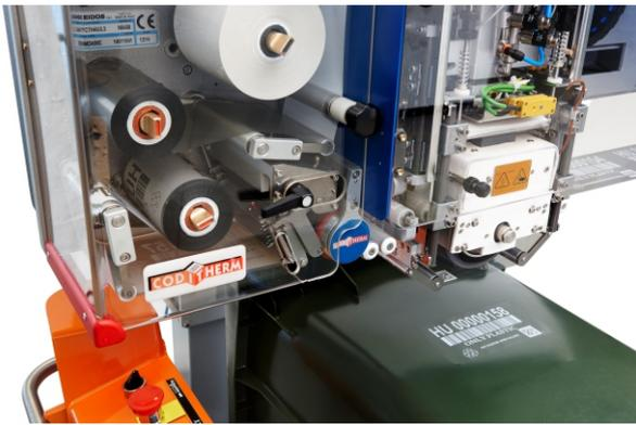
In over 40 years of business, Eidos has developed and patented the procedure for direct thermal transfer printing on solid objects.
