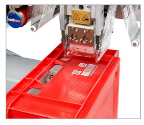
The new high thermal energy Coditherm printers are also able to print inside recessed areas of plastic containers.
